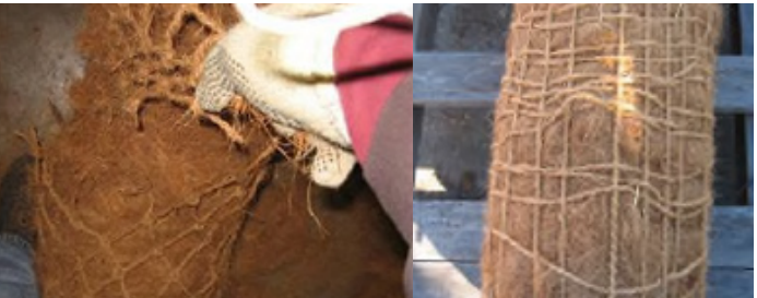
Attempt to Compact 12” Natural Coir Net to 9 lbs/ft³ Density Inconsistent Netting
