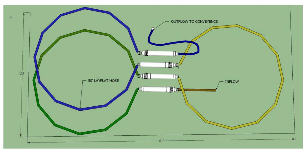
Compact setup with increased contact and mix time. (The total number of Floc Hogs can be adjusted based on need. This is an example only)
