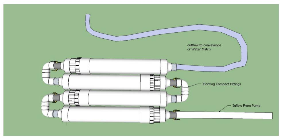
Compact Setup with Water Matrix example. If used with the Water Matrix, 50' of discharge hose is not required after Flog Hog discharge. (The total number of Floc Hogs can be adjusted based on need. This is an example only)
