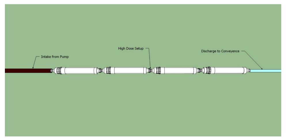
Parallel For use with large greater than 500 GPM pumps: (The total number of Floc Hogs can be adjusted based on need. This is an example only). The split manifold shown is not to scale or accurate of the many types available.
